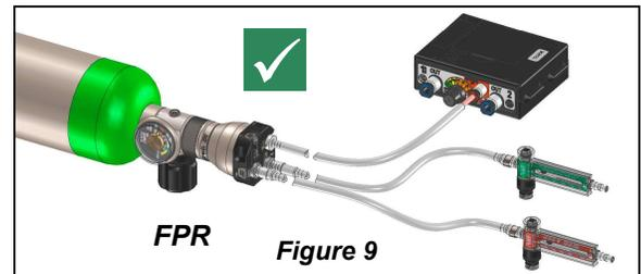
Use the XCP-to-EDS Supply Adapter tubing (00EDS-1070-00) that came with your EDS unit to connect the EDS to the FPR. MH3 and MH4 constant-flow devices connect directly to the CPC connector ports on the FPR regulator.
