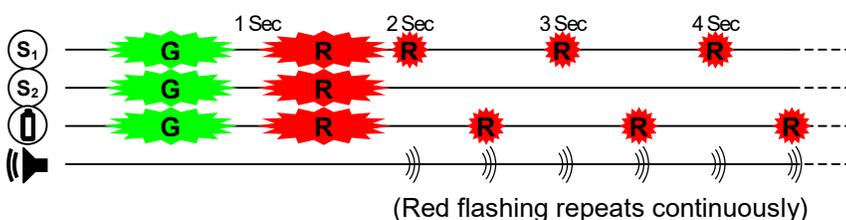
Battery Warning LED and Station LED alternately flash **Red** accompanied by a high chirping tone. The batteries are too low to operate the EDS unit and it will not dispense oxygen.
