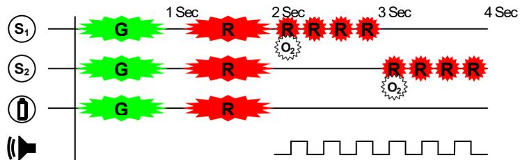
The oxygen pulse will be evident from the sound of the valve opening, or if you have donned your cannula, you will be able to feel the pulse in your nostrils. See **OXYGEN SYSTEM PRE-FLIGHT**, page 12.
