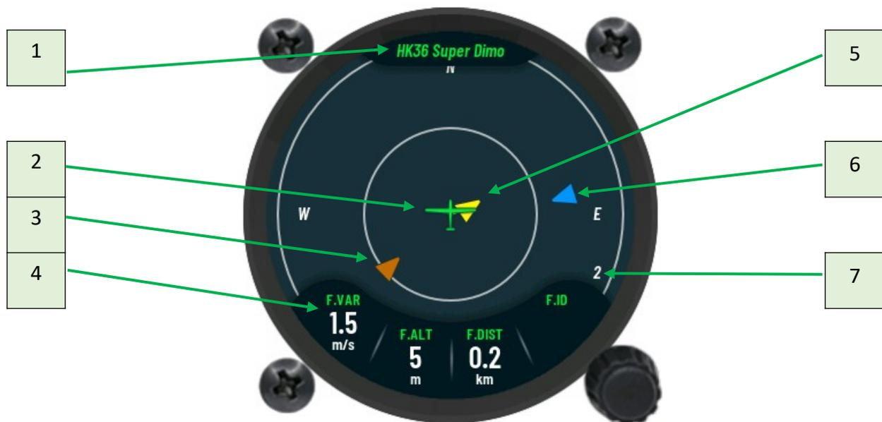
Figure 3: Flarm Radar reference .
