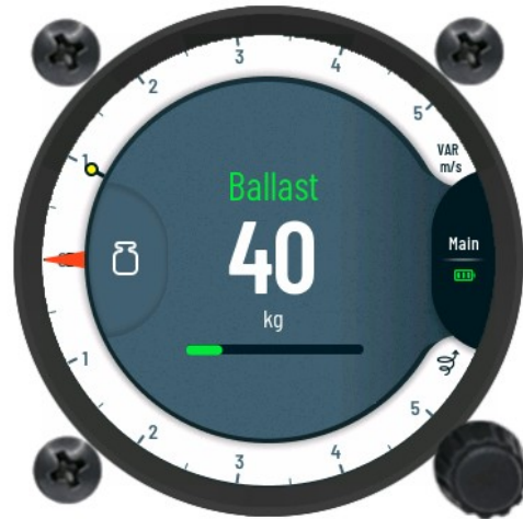
Figure 16: Ballast set view.
