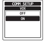
The "\undbelow" icon, which indicates that the VOX system is active, will appear at the right side of the channel frequency when the display returns to the COM band screen.
