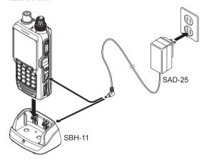
3. Insert the transceiver into the **SBH-11**; the antenna jack should be at the left side when viewing the cradle from the front.
