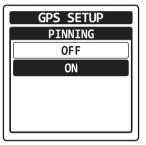
Turning on/off the differential GPS feature You may use the SBAS (satellite-based augmentation system) while obtaining the position information.
