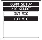
When an optional aviation headset is connected, the **PTT** switch on the radio will activate the headset microphone for transmission.
