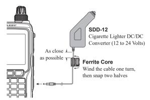
O For noise reduction from exogenous noise, wind one turn of the **SDD-12** cable around the ferrite core, and snap its two halves together, per the illustration
