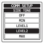
☐ To change the side tone level temporarily during the monitoring, rotate the **DIAL** selector knob when pressing and holding the PTT switch.
