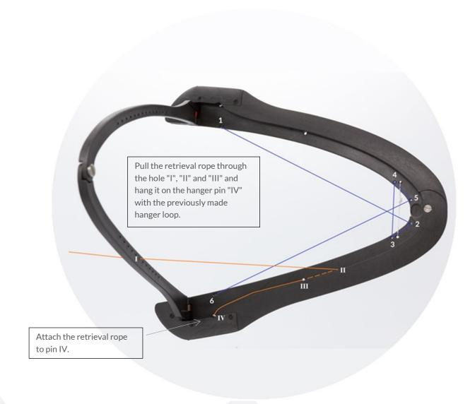
PICTURE 9: HOOKING IN THE RETURN ROPE
